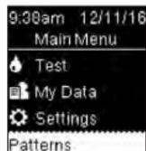
Turn the meter on by briefly pressing **OK**. From **Main Menu**, press **▼** to highlight the Patterns option at the bottom of the screen (the example here is **Patterns**). Press **OK**.
