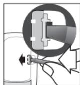
Open the child-resistant battery door by inserting a narrow object, such as a pen, into the slot. Push the tab in the direction of the arrow and lift the battery door up.
