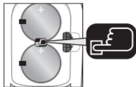
Release the old batteries by pressing the
