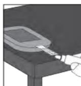
Touch the drop to the **yellow edge** of the test strip. Do not put control solution on top of the test strip.
