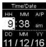
Press **▼** or **▲** to adjust each field. Press **OK** to set and move to the next field. Set **am** or **pm** if necessary.
