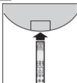
Insert the metallic end of the test strip into the meter.
