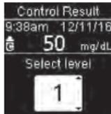
**Control Result** and the control bottle symbol appear. Press  $\blacktriangledown$  or  $\blacktriangle$  to select the control level you tested. If you do not select a level, the control result is saved without a control level. Press **OK**.
