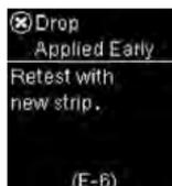
Blood or control solution was applied to the test strip before **Apply drop** appeared.
