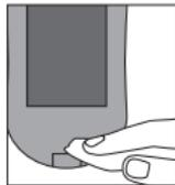
Turn the meter off and wipe the entire meter surface with a Super Sani-Cloth. Carefully wipe around the test strip slot and other openings.
