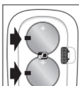
Slide the new batteries under the black tabs and the
