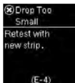
Not enough blood or control solution was drawn into the test strip for measurement or was applied after the test had started.
