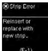
The test strip may be damaged, not properly inserted, or was previously used.
