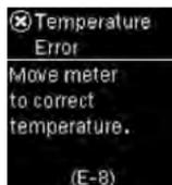
The temperature is above or below the proper range for the system.
