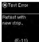
The test strip may be damaged.
