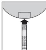
Insert the metallic end of the test strip into the meter. Place the meter on a flat surface.
