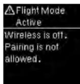
Pairing to a pump cannot be performed while in Flight Mode.
