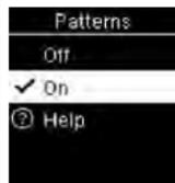
Press **▼** to highlight **On**. Press **OK** to move **✓** to the option. Press **OK**.
