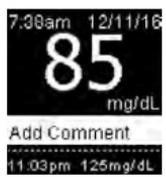
After performing a blood glucose test, the test result is displayed on the screen with **Add Comment** highlighted. Press **OK** to add a comment.
