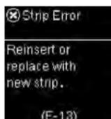
Fluid or foreign material may be present in the test strip slot.
